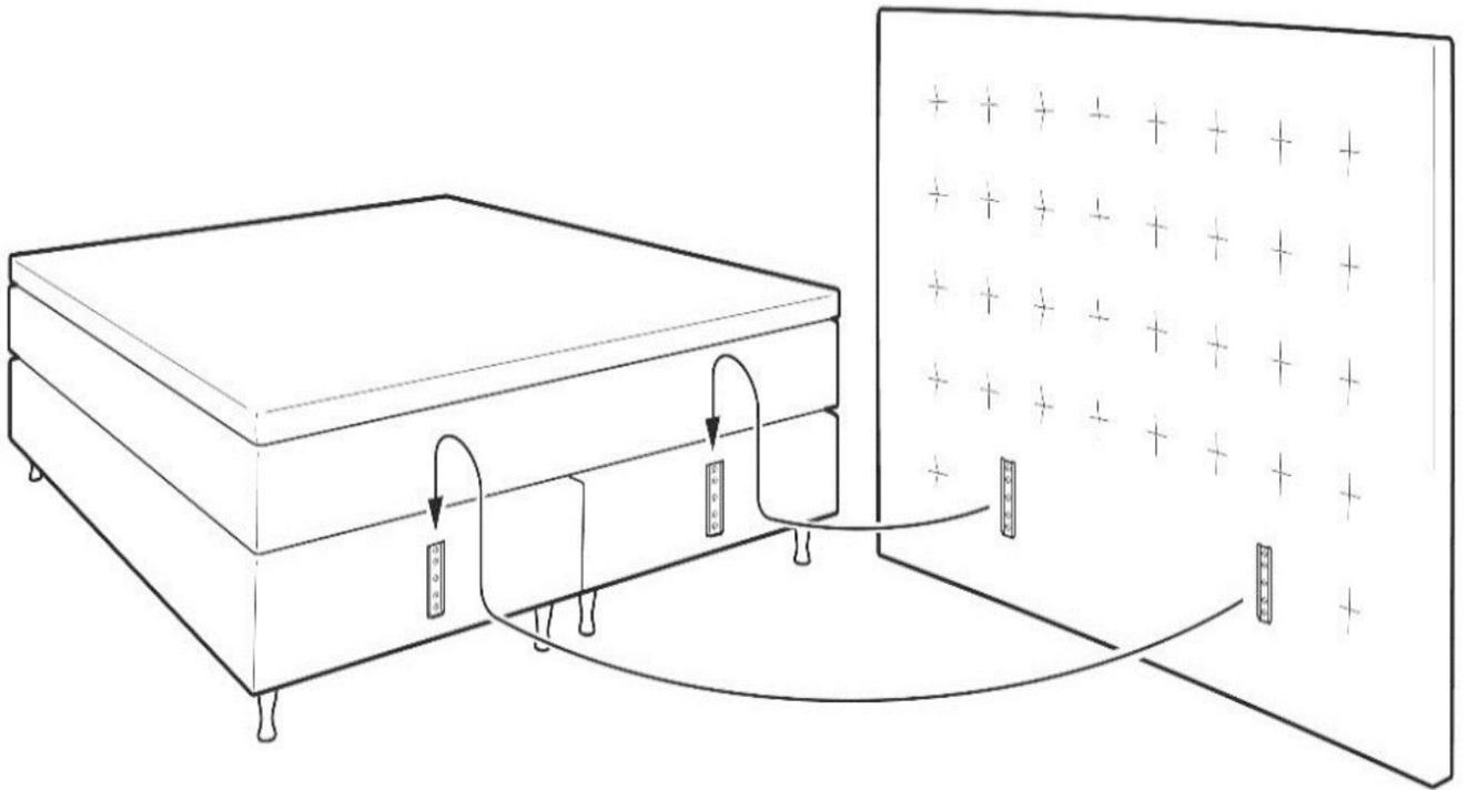
A “U” shaped clip can be used to clip two box springs together to make sure that they don’t separate, see figure 2.
